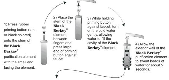
5) Rinse process dust from exterior of purification element. The element has now been successfully primed. Repeat steps 1 - 5 for each additional element.
